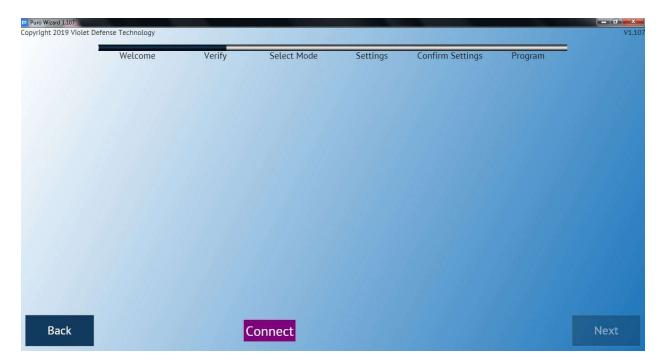
Click on the Verify button on the bottom to confirm connection with your Puro device.
