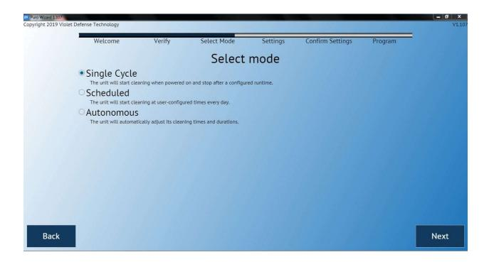
First option is Single Cycle Mode – this option is for single uses of your Puro devices, meaning you will plug it in or turn the switch on each time you want it to run. You can choose between 15 and 30 minute cycles, and you can choose the time it take to start after detecting no motion. Click on Next to proceed.
